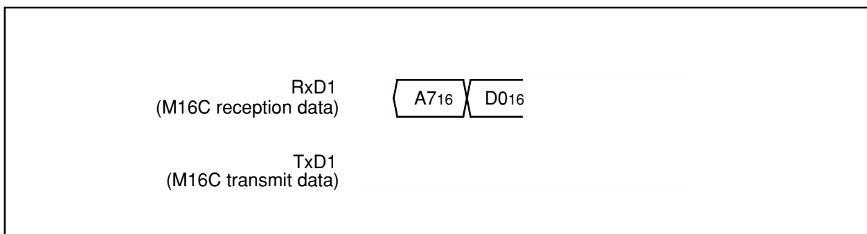
Figure 1.32.27. Timing for erasing all unlocked blocks
