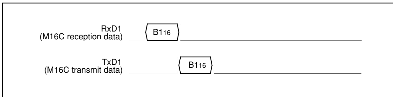
Figure 1.32.39. Timing of baud rate 19200
